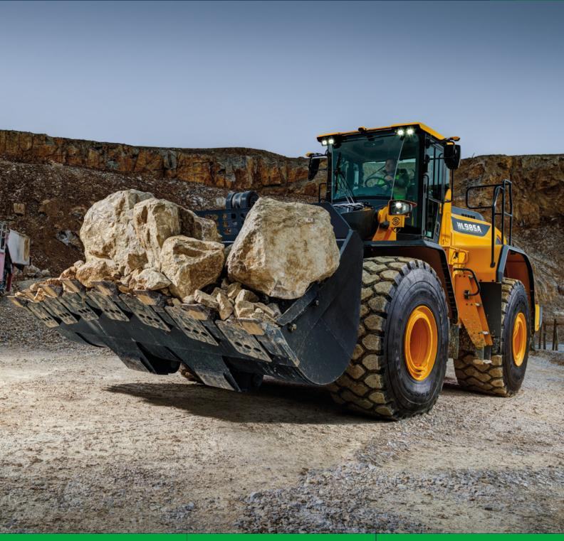
Engine Power 430 HP (321 kW) 2100 rpm Bucket Capacity 6.5 – 7.0 m<sup>3</sup> Operating Weight 33800 kg
